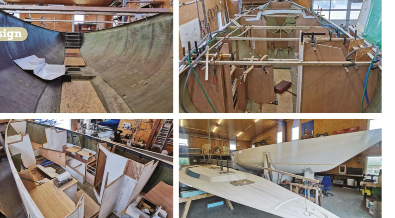
After the initial moulding of hull and deck, the boats are put together and finished at Müritz Bootsservice in Germany
