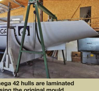
The new Omega 42 hulls are laminated in Sweden using the original mould
